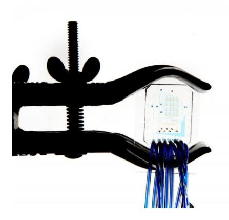
It is possible to load the blood sample directly onto the device and to perform onchip biomarker quantitation without requiring any sample pre-treatment. Credit: Alban Kakulya
