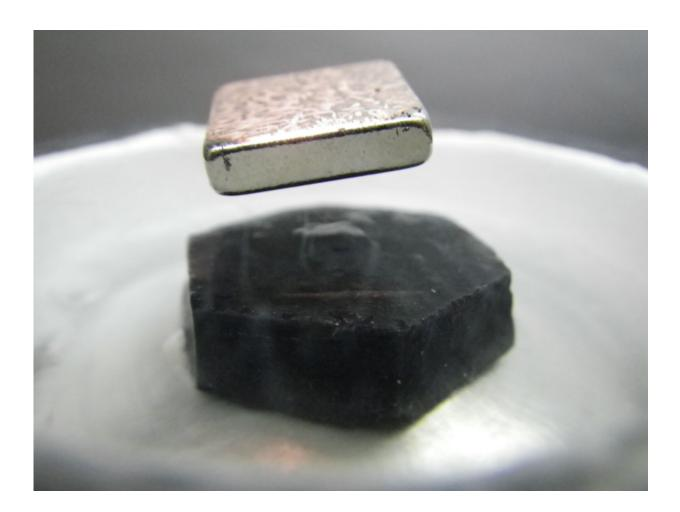
A magnet levitating above a cuprate high temperature superconductor. New findings from an international collaboration led by Canadian scientists may eventually lead to a theory of how superconductivity initiates at the atomic level, a key step in understanding how to harness the potential of materials that could provide lossless energy storage, levitating trains and ultra-fast supercomputers. Credit: Robert Hill/University of Waterloo
