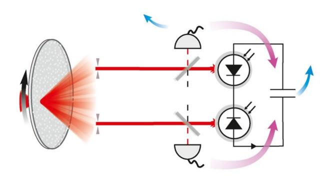
Experimental setup of the photonic Maxwell's demon: The demon's measurement is implemented by high transmittance beam splitters (BS) and highly sensitive avalanche photodiodes (APDs). The two photodiodes are the work extraction mechanism that use the imbalance in the pulse energies created by the demon to charge a capacitor. Credit: Vidrighin, et al. ©2016 American Physical Society
