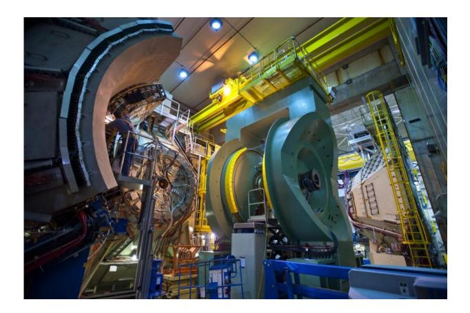
The PHENIX detector at the Relativistic Heavy Ion Collider (RHIC), a particle accelerator at Brookhaven National Laboratory uniquely capable of measuring how a proton's internal building blocks — quarks and gluons — contribute to its overall intrinsic angular momentum, or "spin."
