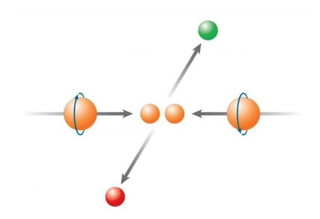
RHIC is the only machine in the world that can collide protons with their spins aligned in a particular direction. Measuring differences in the particles produced when the spins in the two beams are pointing at one another (as shown) vs. when they are pointing in the same direction, colliding "head" to "tail," can help scientists tease out the contribution made by gluons.
