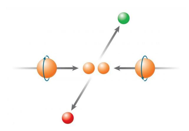
RHIC is the only machine in the world that can collide protons with their spins aligned in a particular direction. Measuring differences in the particles produced when the spins in the two beams are pointing at one another (as shown) vs. when they are pointing in the same direction, colliding "head" to "tail," can help scientists tease out the contribution made by gluons.
