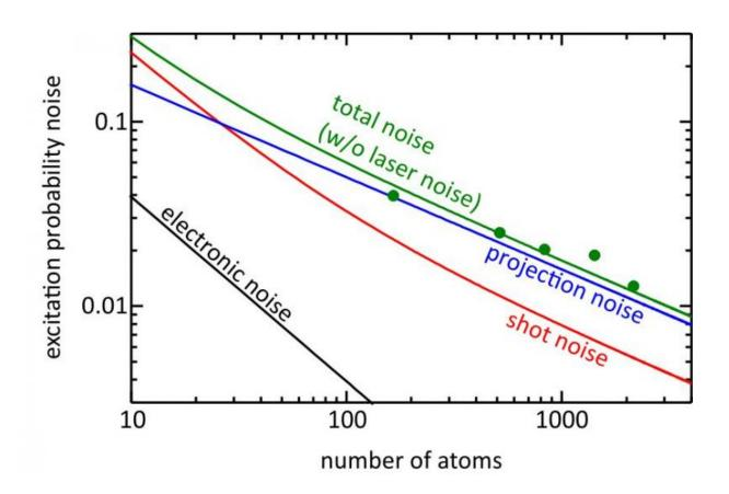
Noise contributions of the strontium lattice clock as a function of the number of atoms. The predicted total noise at suppressed frequency noise of the interrogation laser (green line) is confirmed by experimental data (green circles). The quantum projection noise (blue line) already dominates with few atoms. Credit: PTB
