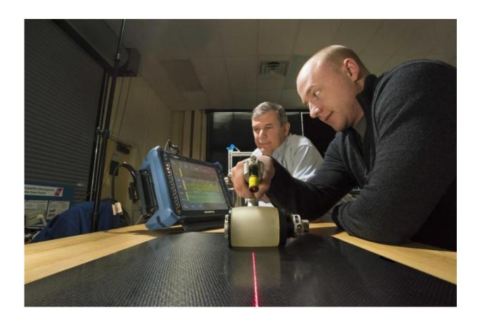
andia National Laboratories technologist Andrew Lentfer passes a roller probe over a composite as researcher David Moore checks data on a screen. The nondestructive testing technique sends sound waves into the composite material, returning data with each swipe of the roller probe. Credit: Randy Montoya
