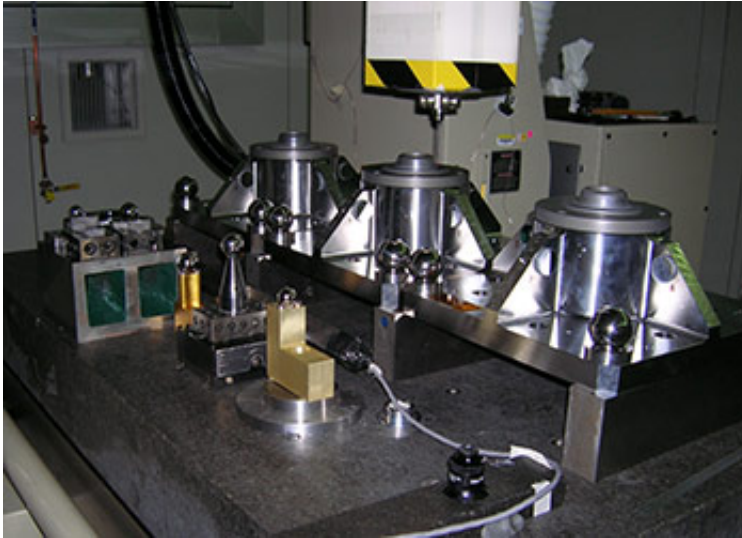
Three of the four James Webb Space Telescope Primary Mirror Backplane Support Structure fixtures on the NIST M48 Coordinate Measuring Machine. Credit: John Stoup/NIST
