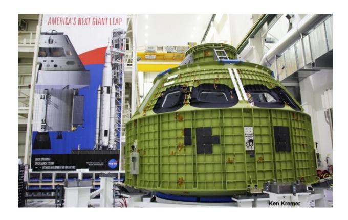
Orion crew module pressure vessel for NASA's Exploration Mission-1 (EM-1) is unveiled for the first time on Feb. 3, 2016 after arrival at the agency's Kennedy Space Center (KSC) in Florida. It is secured for processing in a test stand called the birdcage in the high bay inside the Neil Armstrong Operations and Checkout (O&C) Building at KSC. Launch to the Moon is slated in 2018 atop the SLS rocket. Credit: Ken Kremer/kenkremer.com
