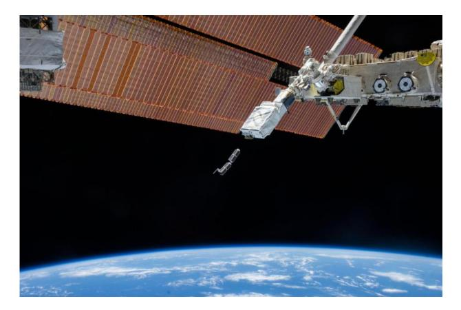
In February 2014, Planet Labs Inc. launched its first flock of Dove nanosatellites into space. Shown are two shoebox-sized Doves being ejected into low-Earth orbit from the International Space Station. The company's goal is for the flock to take a high-resolution snapshot of nearly the entire globe every 24 hours. Credit: NASA
