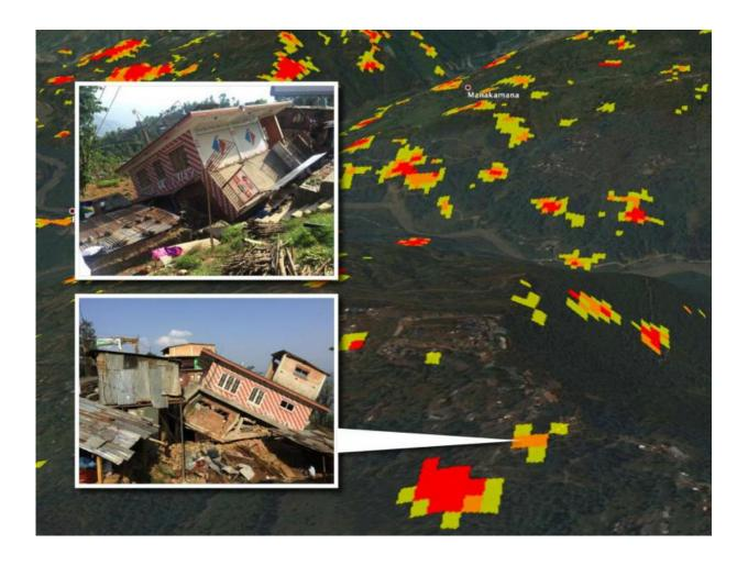
Street-level photos from locations on a mountain ridgetop in Nepal are overlaid on a damage proxy map derived from data from the ALOS-2 satellite. The color gradation represents increasingly more significant change on the ground, with red being the most severe and yellow being the least severe. Credit: NASA/JPL-Caltech/Google/DigitalGlobe/Amy MacDonald/Thornton Tomasetti
