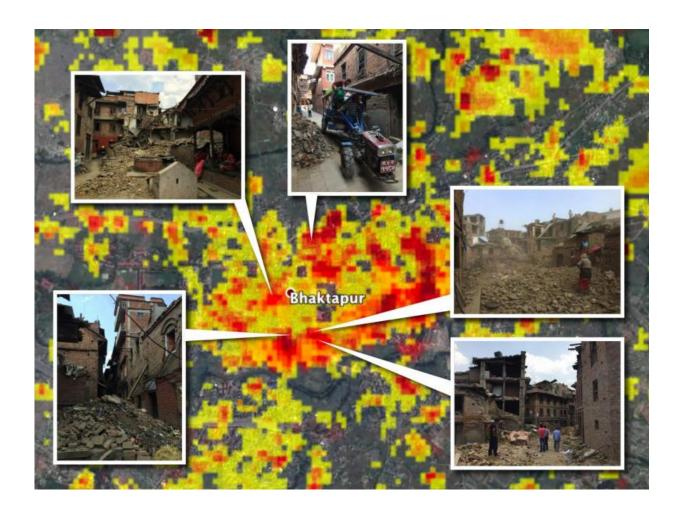
This image shows street-level photos in the Bhaktapur area of Nepal overlaid on a damage proxy map derived from data from COSMO-SkyMed satellites. The color gradation -- yellow to orange to red -- represents increasingly more significant change on the ground. Credit: NASA/JPL-Caltech/Google/DigitalGlobe/CNES/Astrium/Amy MacDonald/Thornton
