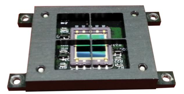
A closeup of the Wallops-developed fine sun sensor that is flying on the CANYVAL-X mission. Credit: NASA
