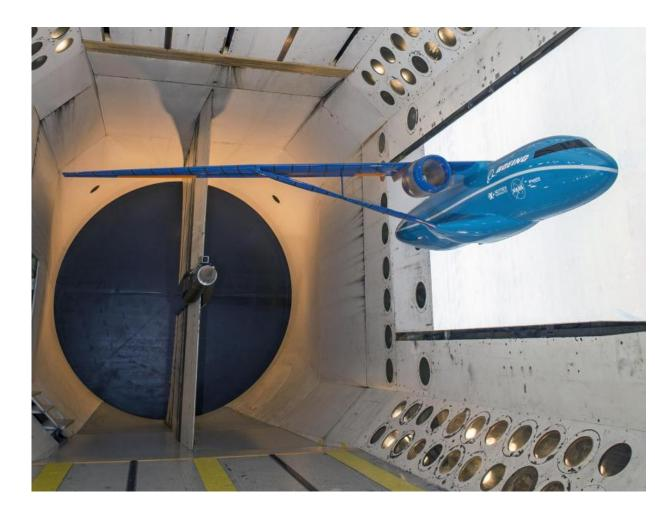
This truss-braced wing concept could be another subsonic X-plane; the supported wing has proven in wind-tunnel testing to reduce fuel use by 5 to 10 percent over advanced conventional wings. Credit: NASA Langley / Sandie Gibbs
