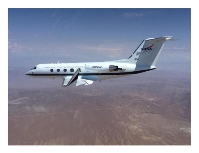
One tech demo successfully completed tests of flaps that can be changed to different angles during flight, reducing drag and noise. Credit: NASA
