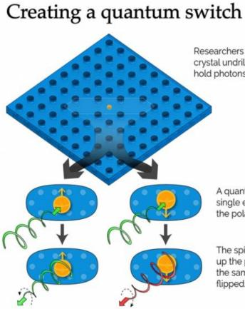
Researchers leave several holes in a photonic crystal undrilled, creating a cavity that can hold photons.
