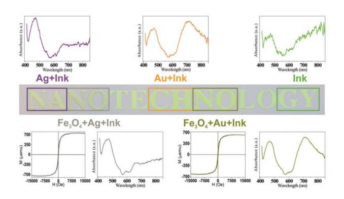
A paper with the word "Nanotechnology," where different pairs of letters are printed with different combinations of overlapping nanoparticle inks. Credit: Campos-Cuerva, et al. ©2016 IOP Publishing
