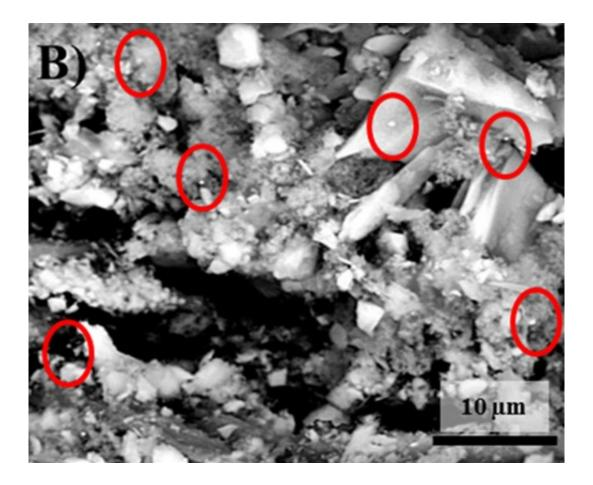
An SEM micrograph of paper printed with nanoparticle-based ink, with the nanoparticles circled in red. Credit: Campos-Cuerva, et al. ©2016 IOP Publishing
