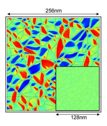
In nanocrystalline shape memory alloys, martensitic transformation (red and blue areas) is suppressed as the grain size decreases (inset) due to grain boundary effects. Credit: AIP Publishing LLC
