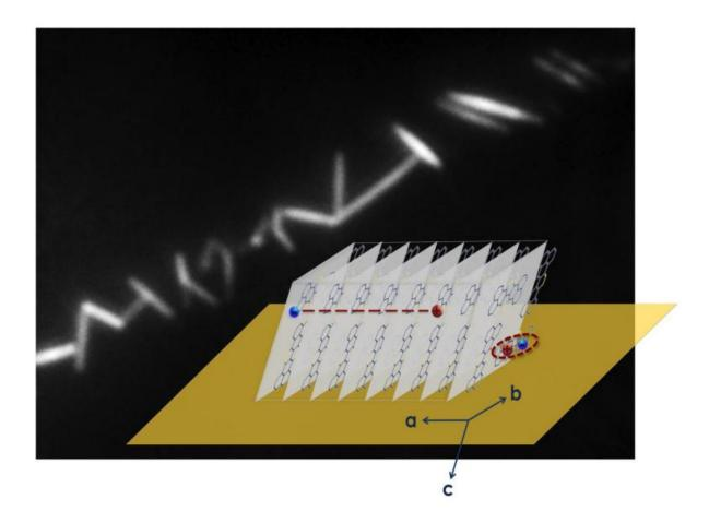
A new paper from UMass Amherst describes a structure that will make it easier to use a certain molecule for new applications, for example in devices that use polarized light input for optical switching, by exploiting its directionality. Inset shows a structural schematic of the TAT crystal packing geometry and direction of charge separation. Credit: UMass Amherst/Mike Barnes
