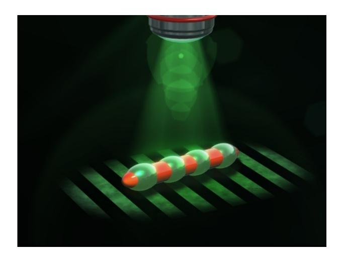
Light-driven microswimmers: the material of the swimming body, which measures just under one millimetre in length, is chosen so that it changes shape when exposed to green light. This causes wave-shaped protrusions to form along the swimmer and drive it in the opposite direction when light patterns move over its surface. Credit: Alejandro Posada
