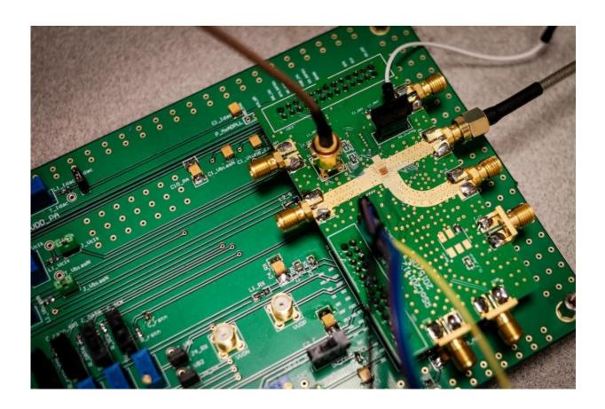
NTU's tiny microchip for radar imaging embedded on a PCB board (small square chip on the upper right)
