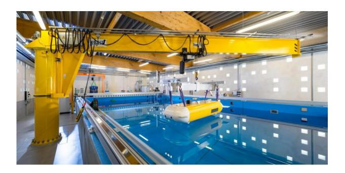
The underwater vehicle suspended above the maritime systems research platform with its slewing crane, portal system and (in the background on the left) pressure chamber. Credit: Fraunhofer IOSB-AST
