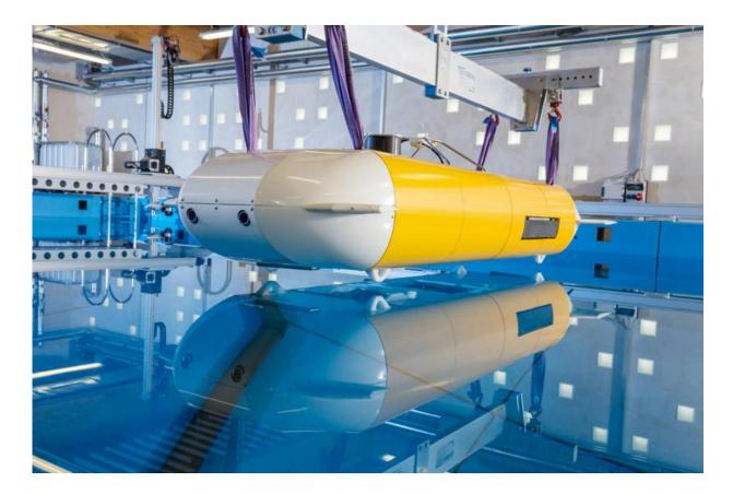
The AUV weighs less than 700 kilograms, making it a truly lightweight vehicle.
