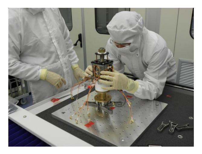
Assembly of one of the Inertial Sensor Heads for the LISA Technology Package (LTP). Credit: CGS SpA
