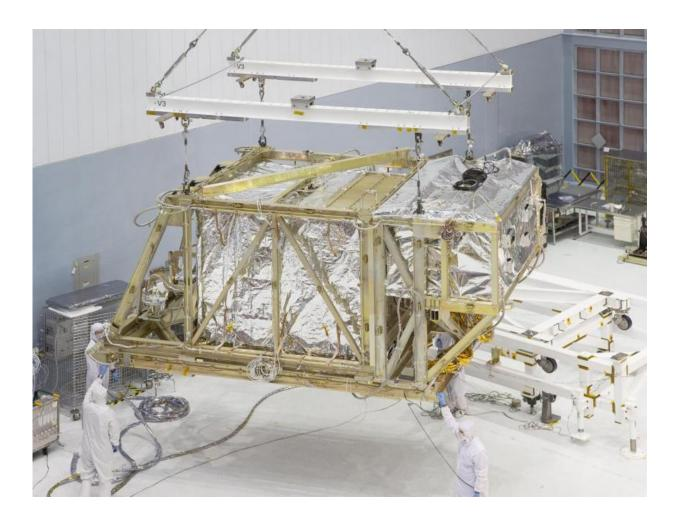
Moving the JWST Integrated Science Instrument Module (ISIM) from a clean room at the Goddard Space Flight Centre to the Space Environment Simulator for the third long-duration cryo-vacuum test, known as ISIM CV-3. Credit: NASA/Chris Gunn
