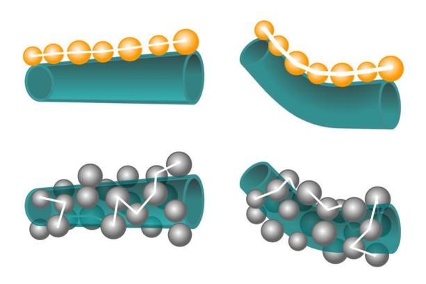
Iron-dotted boron nitride nanotubes, made in Yoke Khin Yaps' lab at Michigan Tech, could make for better wearable tech because of their flexibility and electronic behaviors. Credit: Michigan Tech, Sue Hill
