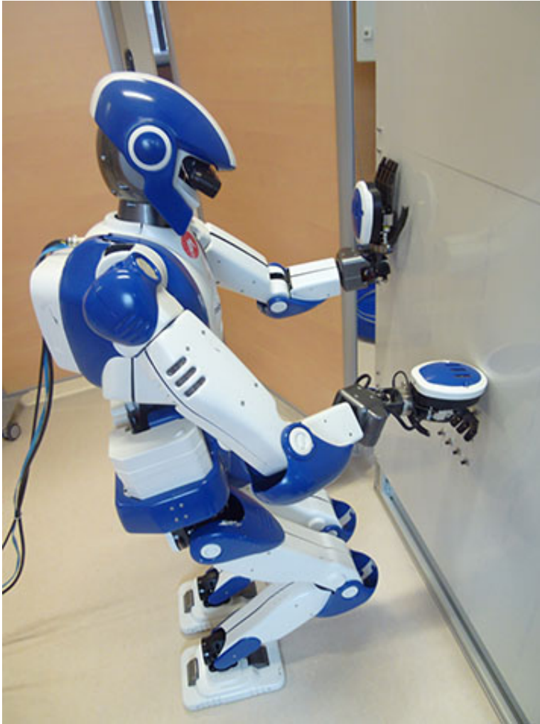
Planning and control of multi-contact movements by humanoid robots. Credit: Joint Robotics Laboratory (CNRS/AIST)
