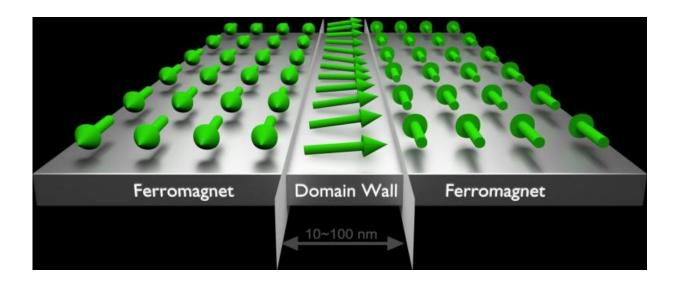
The spin wave remains trapped in the domain wall, which is formed in the middle between the differently oriented magnetizations. Researchers at the HZDR could thus control its propagation purposefully. Credit: HZDR / H. Schultheiß
