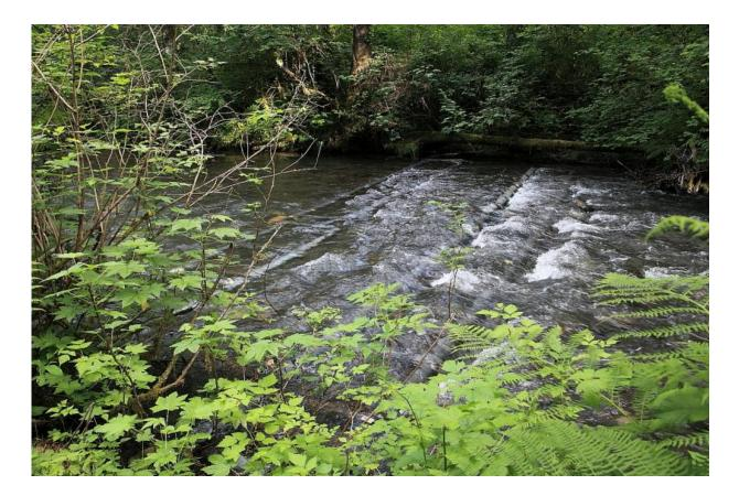
Antennas embedded in a Washington stream bottom help measure how fish use restored habitat in an intensively monitored watershed. The parallel antennas are visible as the water flows over them. Credit: John McMillan, NOAA Fisheries/NWFSC
