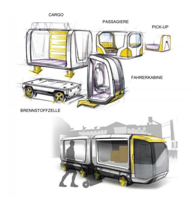
The Citylog EMF (Electronic-mulit-funktion-vehicle) consists of single wagons that can be linked together, each with a motor and fuel cell energy supply. Each wagon has a total weight of 2000 kg, with the first wagon incorporating a driver's cabin. Credit: HET Engineering
