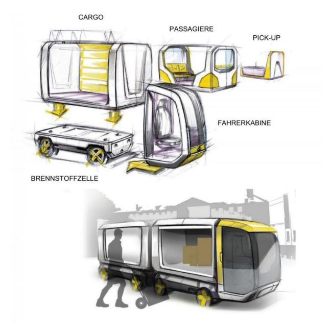
The Citylog EMF (Electronic-mulit-funktion-vehicle) consists of single wagons that can be linked together, each with a motor and fuel cell energy supply. Each wagon has a total weight of 2000 kg, with the first wagon incorporating a driver's cabin. Credit: HET Engineering
