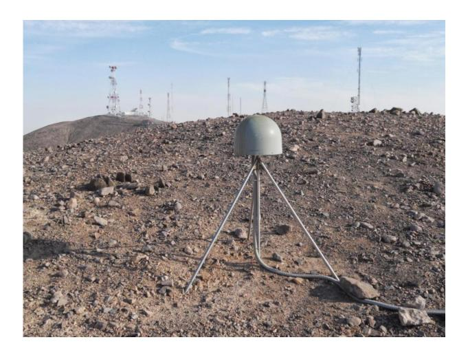
An example of a scientific GPS instrument used at monitoring stations. The instrument is perfectly mounted to the ground, and can measure motions as small as half an inch, or the size of a quarter. By contrast, phone GPS can only approximate your location within a meter (or a few feet) of your exact location. Photo taken in Chile. Credit: Sebastian Riquelme
