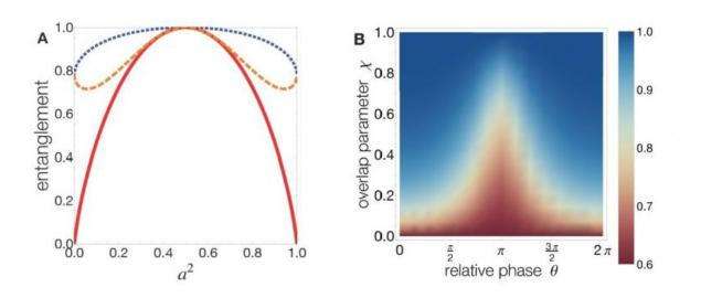
(Left) A comparison of entanglement for nonidentical particles (red solid line) with identical bosons (blue dotted line) and identical fermions (orange dashed line). (Right) Density plot of entanglement for identical bosons, which—unlike nonidentical particles—depends on particle overlap. Credit: Lo Franco and Compagno. ©2016 Nature *Scientific Reports*
