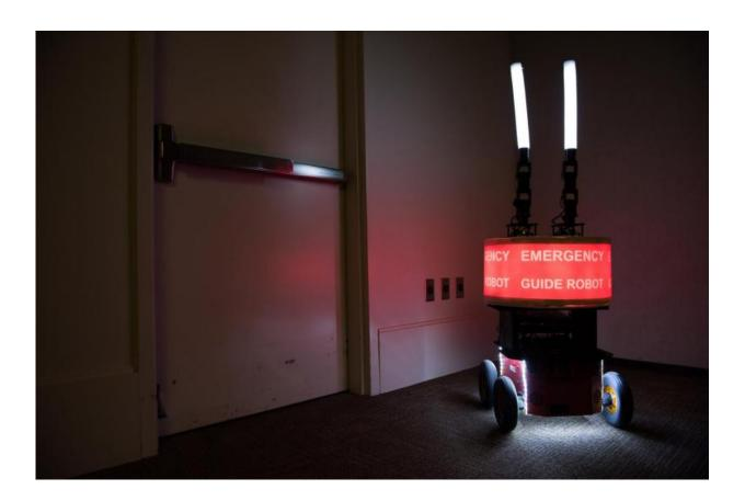
Georgia Tech researchers built the 'Rescue Robot' to determine whether or not building occupants would trust a robot designed to help them evacuate a high-rise in case of fire or other emergency. Credit: Rob Felt, Georgia Tech
