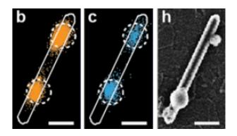
Flashes of fluorescence seen under a microscope show where chemical reactions to (b) split water molecules or (c) electric currents take place on a nanorod of photovoltaic material. The outline of the rod laid over flash images is taken from the scanning electron microscope image at right.
