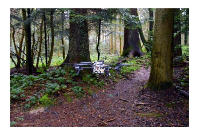
Using a new software drones detect forest paths and can follow these autonomously. Credit: UZH; USI; SUPSI
