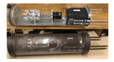
Newer version of the device known as the IS2B. The tool is a kind of mobile laboratory or pod for performing precision analysis on sampled water and sediment. Credit: The Biodesign Institute
