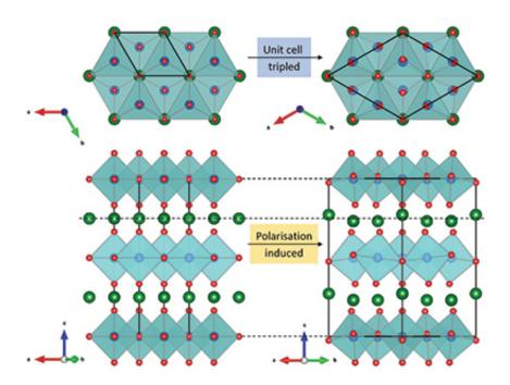
Crystal structures of paraelectric and ferroelectric phases. Credit: Sim et al.
