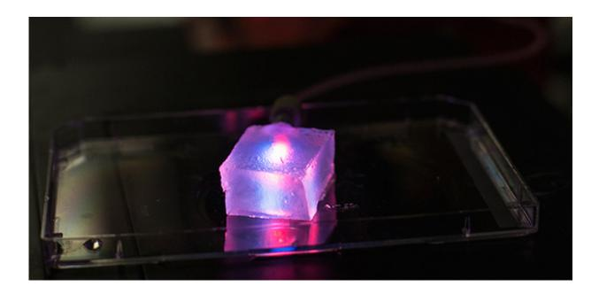
Three-dimensional slab of gelatin that contains a microvascular network. Credit: Bellan Lab / Vanderbilt
