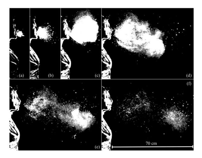
This sequence illustrates the evolution of the multiphase turbulence cloud that suspends droplets emitted during a sneeze. Shown here are times ranging from 7 to 340 milliseconds post sneeze onset. Credit: From the paper, "Visualization of sneeze ejecta: steps of fluid fragmentation leading to respiratory droplets," by B. E. Scharfman, A. H. Techet, J. W. M. Bush, L. Bourouiba.
