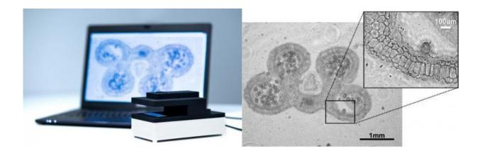
At next week's SPIE Photonics West 2016, imec will demonstrate a lensfree microscope for large field-of-view live imaging at micrometer resolution. Imec's on-chip lens-free microscope can be integrated into life sciences and biotech tools, targeting multiple applications such as label-free cell monitoring, automated cell culturing, or automated highthroughput microscopy.
