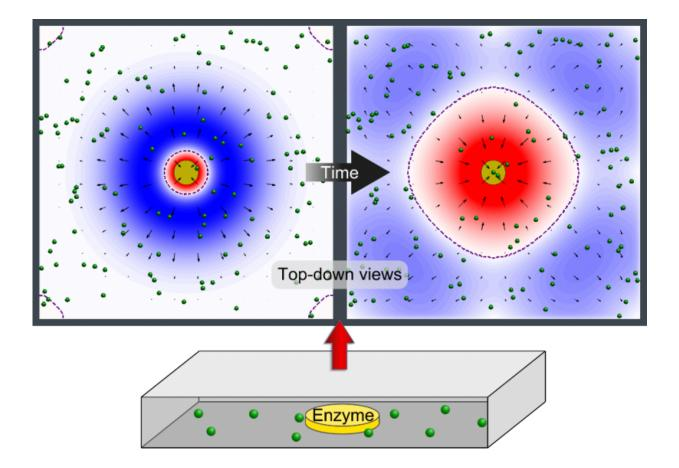
A patch of enzymes immobilized on a surface acts as a fluid pump. Fluid, and small particles (green spheres) carried by the fluid, can be simultaneously pumped away from the patch (blue) in some parts of the chamber and toward the
