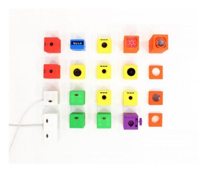
Cambits, a modular imaging system that can transform into many different cameras, has been developed by Columbia Engineering Computer Science Professor Shree Nayar and Makoto Odamaki, visiting scientist from Ricoh Corporation. Credit: Shree Nayar/Columbia Engineering
