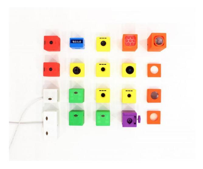
Cambits, a modular imaging system that can transform into many different cameras, has been developed by Columbia Engineering Computer Science Professor Shree Nayar and Makoto Odamaki, visiting scientist from Ricoh Corporation. Credit: Shree Nayar/Columbia Engineering
