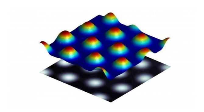
Exploiting cellular convection in a thick liquid layer to pattern a polymer film is pictured. Credit: Iman Nejati/TU Darmstadt
