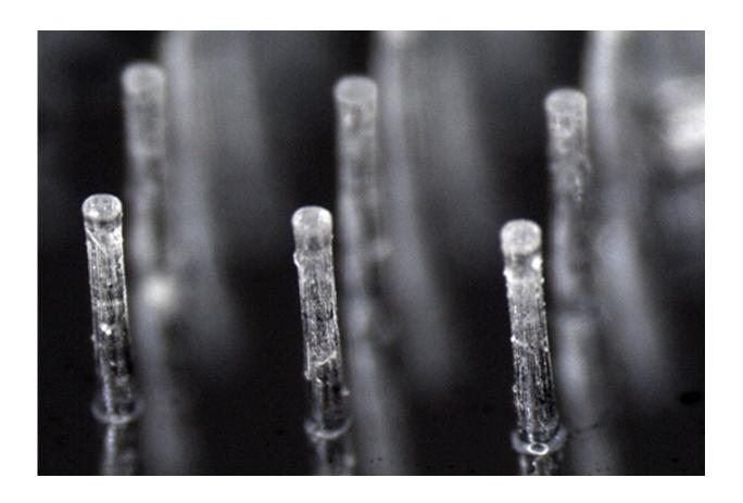
A close-up image of micro-scale pillars that were formed — or, photostructured — in the OSTE polymer using UV light. Credit: KTH Royal Institute of Technology
