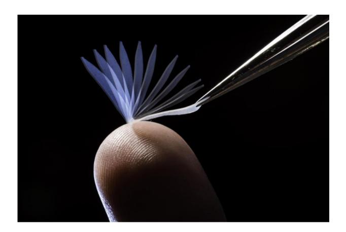
A time-lapse photo of a new shape-memory polymer reverting to its original shape after being exposed to body temperature. Credit: Adam Fenster/University of Rochester
