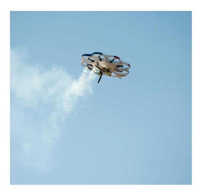
Drone America's DAx8 multi-rotor aircraft deploys two cloud seeding flares
