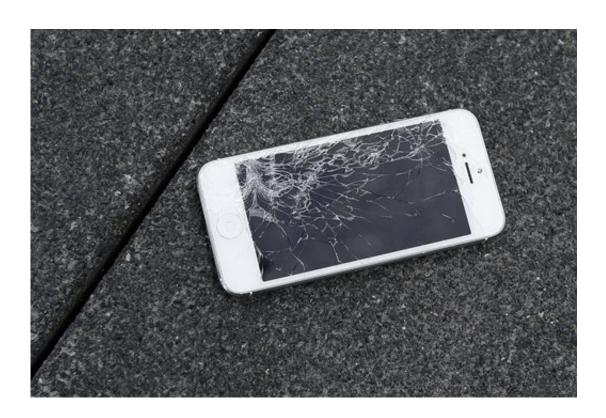
This Aug. 26, 2015 photo shows an Apple iPhone with a cracked screen after a drop test from the DropBot, a robot used to measure the sustainability of a phone to dropping, at the offices of SquareTrade in San Francisco. Apple for the first time is accepting banged up iPhones as a trade-in from those wanting to upgrade. (AP Photo/Ben Margot)
