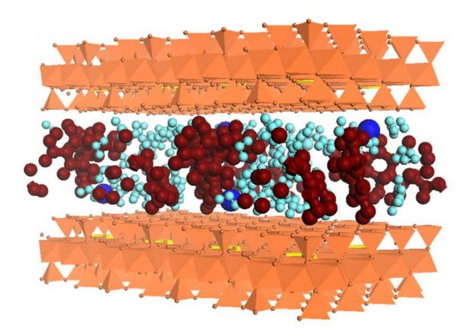
Simulation of clay nanopores containing trapped tetracycline antibiotic compounds: water molecules (light blue), metals (dark blue), antibiotics (dark red), clay layer (orange), negative charges in clay structure (yellow). Credit: Ludmilla Aristilde
