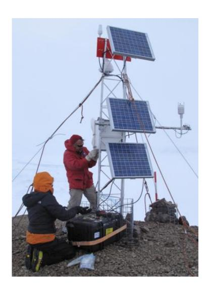
NSIDC lead scientist Ted Scambos and a colleague install a first generation Automated Meteorology-Ice-Geophysics Observing System-I (AMIGOS-I) at Cape Disappointment on the Antarctic Peninsula on November 2011. NSIDC researchers will be testing version 2 of the system (AMIGOS-II) on the frozen surface of Grand Lake, Colorado.
