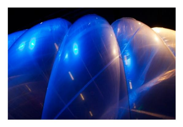
The current design of Project Loon is a balloon within a balloon: one containing helium to keep it aloft and the other with air that can be released or added to move up or down
