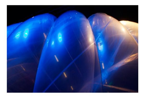
The current design of Project Loon is a balloon within a balloon: one containing helium to keep it aloft and the other with air that can be released or added to move up or down
