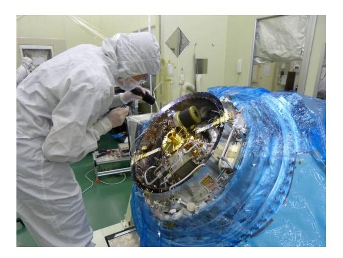
An instrument scientist inspects the Soft X-ray Spectrometer before its final closing. The SXS is one of four payloads flying on the Japanese-led Hitomi mission launching in February. Credit: NASA
