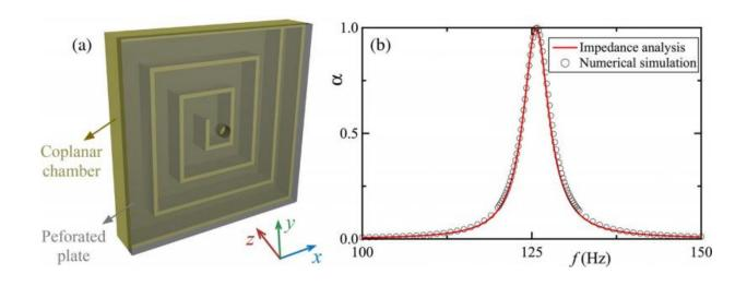
(Left) The metasurface composed of a perforated plate (transparent gray region) with a hole and a coiled coplanar air chamber (yellow region). (right) The absorption coefficient,  $\alpha$ , of the presented metasurface with a total absorption at 125.8 Hz. Results from the impedance analysis and numerical simulations show excellent agreement.
