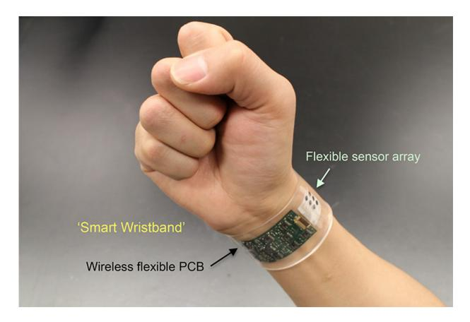
The flexible sensor developed at UC Berkeley can be made into "smart" wristbands or headbands that provide continuous, real-time analysis of the chemicals in sweat. Credit: Wei Gao, UC Berkeley
