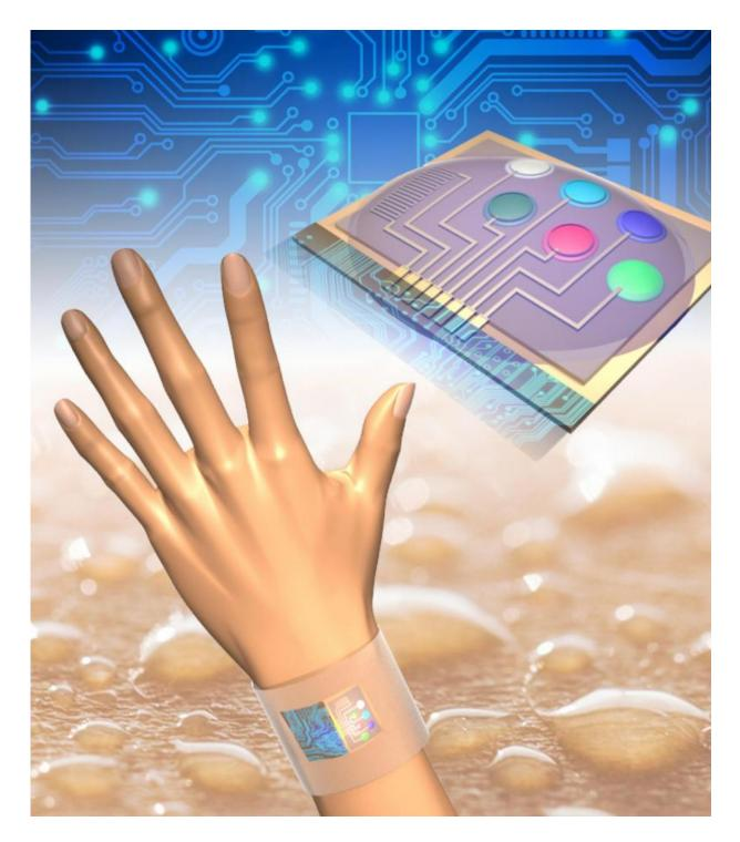
Wearable sensors measure skin temperature in addition to glucose, lactate, sodium and potassium in sweat. Integrated circuits analyze the data and transmit the information wirelessly to a mobile phone. Credit: Der-Hsien Lien and Hiroki Ota, UC Berkeley
