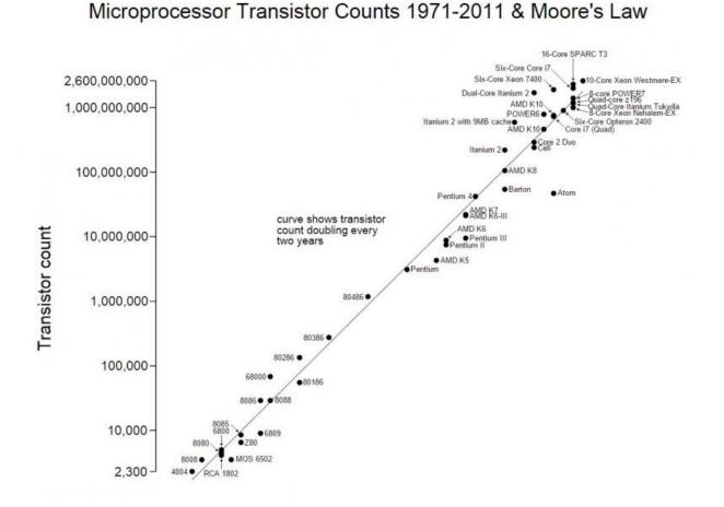
Plot of CPU transistor counts against dates of introduction; note the logarithmic vertical scale; the line corresponds to exponential growth with transistor count doubling every two years. Credit: Wikipedia
